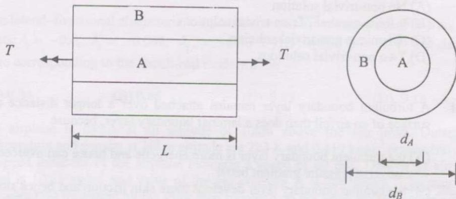
$$(A) \frac{\left(\frac{G_A J_A}{L} \frac{G_B J_B}{L}\right)}{\left(\frac{G_A J_A}{L} + \frac{G_B J_B}{L}\right)}$$
