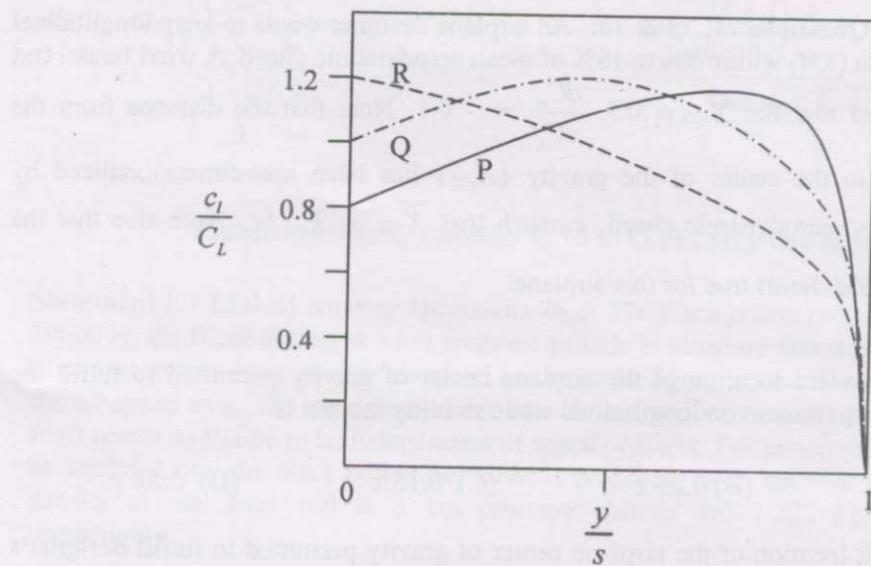
In the above figure,  $c_l$  refers to the section lift coefficient,  $C_L$  refers to the lift coefficient of the wing,  $y$  is the coordinate along the span and  $s$  is the span of the wing. A designer prefers to use a wing for which the stall begins at the root. Which of the wings will he choose?
